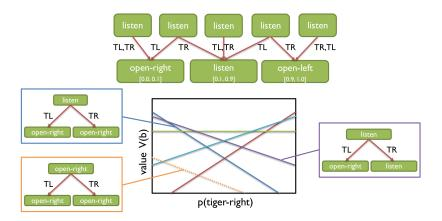
In exact (full) value iteration in POMDPs,  $|V_t| = |\mathcal{A}| \cdot |V_{t-1}|^{|\mathcal{O}|}$ new  $\alpha$ -vectors are generated in each step of the algorithm.
