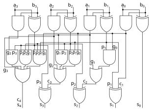
But for two 64-bit inputs, the adder would require  $10^{20}$  gates to be built.
