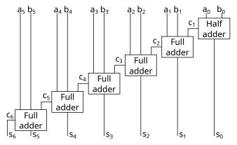
$a_5 a_4 a_3 a_2 a_1 a_0 + b_5 b_4 b_3 b_2 b_1 b_0 = s_6 s_5 s_4 s_3 s_2 s_1 s_0$  where  $s_6 = c_6$
