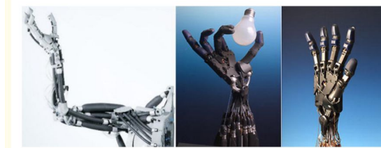
Figure 3. The bionic musculoskeletal robots of the FESTO Airic's arm and the SHADOW hand [5, 6].
