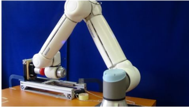
(a) UR10e with AIRSKIN (transient contact).
